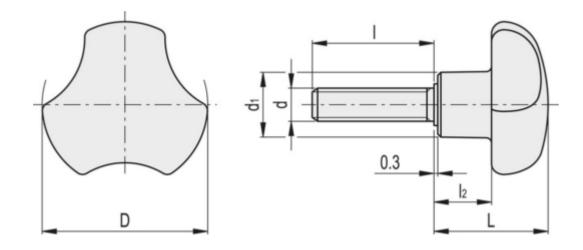
$\begin{array}{lll} D & = 40 \\ d1 & = 16 \\ Dg & = - \\ I2 & = 13.5 \\ L & = 27 \\ L1 & = 30 \\ Weight in (g) = 32 \end{array}$
